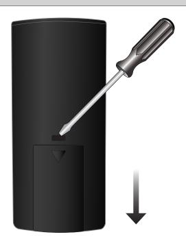
Insert a flat-head screwdriver into the slot as shown. Gently push down on the tab, then press and pull downward on the battery cover to open.
